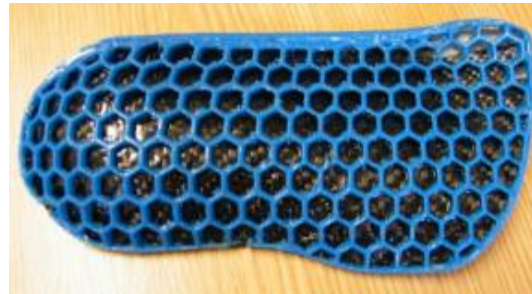
FDM-Made orthotics in PLA with CF reinforcement. a) Top carbon-fibre surface b) lower honey-comb built-time optimized structure
