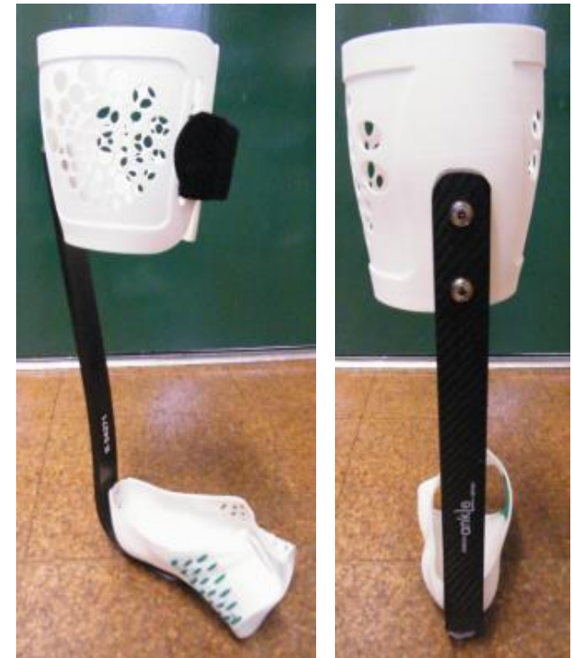
SLS-made AFO in Duraform PA with foot-plate and calf connected by a carbon fibre 7 spring (PCK-UNEW)
