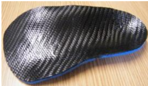
FDM-Made orthotics in PLA with CF reinforcement. a) Top carbon-fibre surface b) lower honey-comb built-time optimized structure
