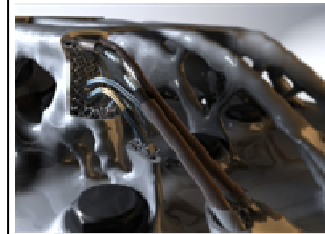
Topologically optimized component with embedded electronic tracks and cooling channels (University of Nottingham)
