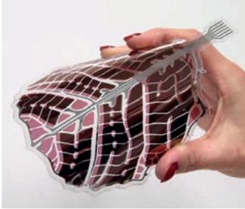
*Decorative solar cell can be used to power battery-less sensors for lighting control. (Source: VTT)*
