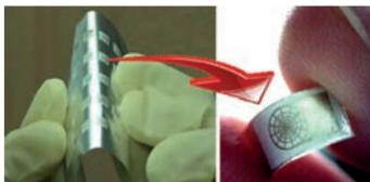
*Thermocouple sensor. (Source: Wang 2010)*
