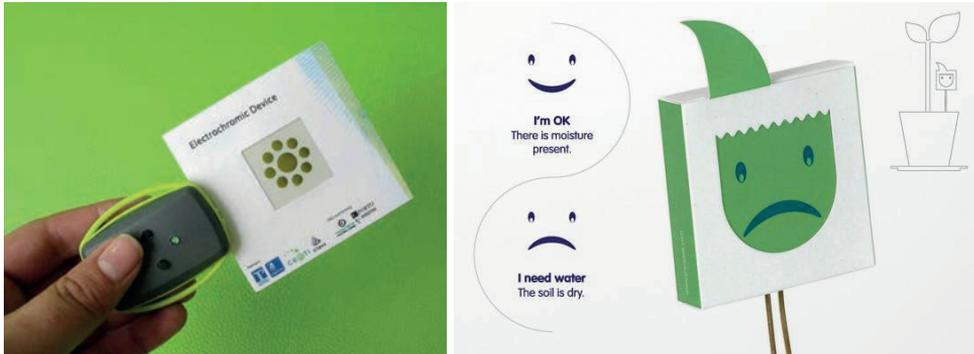
**Figure 3.17.** *Electrochromic Printed Electronics prototypes: free design for customised applications. (Source: CeNTI and Ynvisible)*
