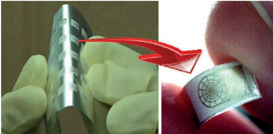
**Figure 3.18.** *Thermocouple sensor. (Source: Wang 2010)*
