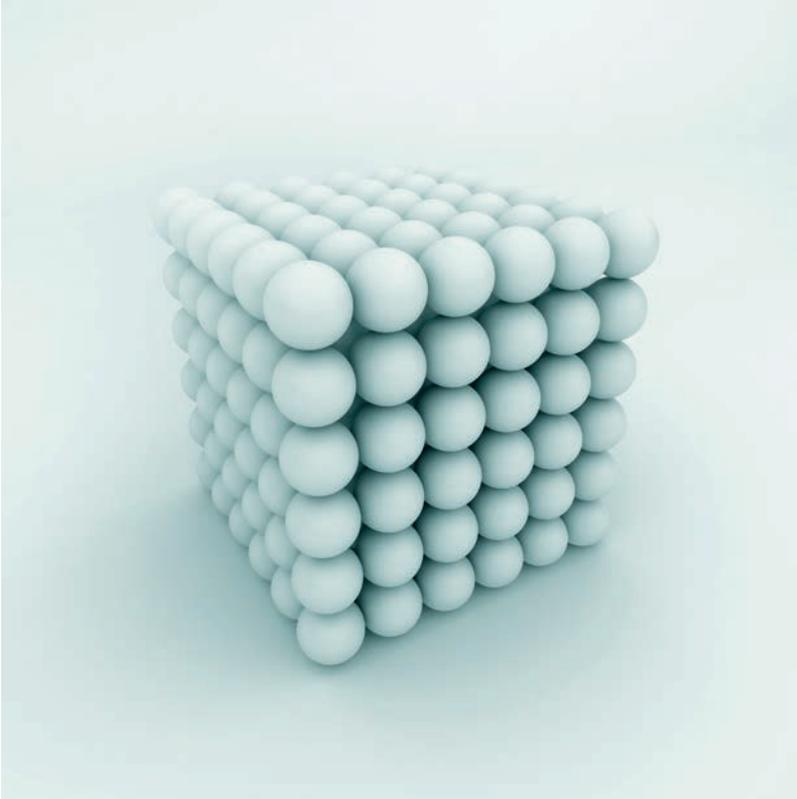
**Figure 3.31.** Artist impression of catoms, the building blocks of the Claytronics concept. Catoms can be programmed individually and interact with each other to form physical 3D objects. (Source: Shutterstock)
