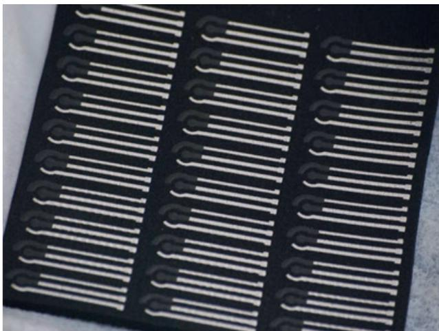
**Figure 3.19.** *Printed electrochemical sensors to detect any contaminants present in seawater, for example: phenols, TNT (trinitrotoluene) and copper. (Developed by the team of Prof. Joseph Wang of UCSD, University of California, San Diego)*
