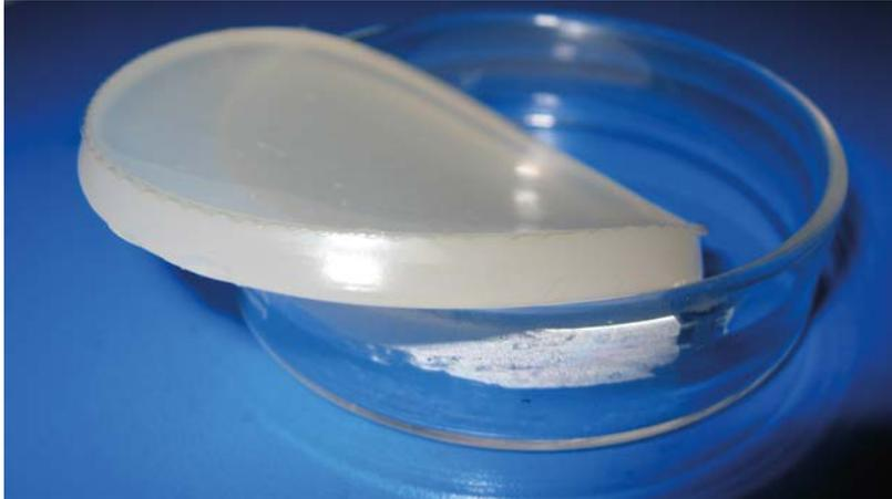
**Figure 3.23.** *Xylan-based hydrogel contains 90 per cent water, but remains mechanically quite durable. (Source: VTT)*
