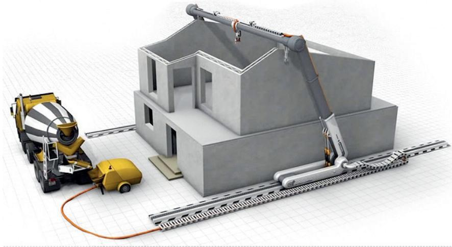
**Figure 3.29.** Artist impression of the so called 'Contour Crafting' technology that enables Digital Fabrication of buildings. (Grozdanic 2014)
