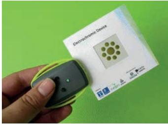
*Electrochromic Printed Electronics prototypes. (Source: CeNTI and Ynvisible)*
