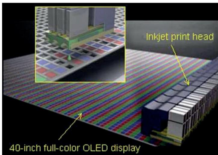
**Figure 3.13.** Schematic representation of inkjet printing for manufacturing of OLED displays. (Digital imageMaker international 2014)
